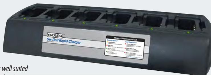
**Endura TWC6M:** With its compact footprint, the TWC6M is well suited for use in an office, shop, or mobile command center. It includes six charging pods that can be configured for a specific radio or six different radios. The TWC6M features an AC to DC external power supply (UL listed) and accessories for in-vehicle installation are also available.
